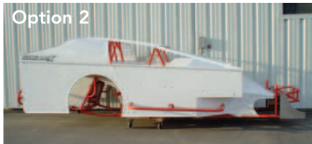
DOM chassis with bumpers, side rails & white body installed
